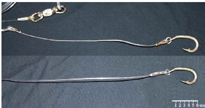
The Hawaii Longline Association proposed switching the Hawai'i deep-set fishery's gear from steel wire leaders (top) to monofilament nylon leaders (bottom) to increase oceanic whitetip sharks and other protected species' chance of survival post-interaction. Wire leaders are commonly used in the industry to increase crew safety by preventing gear flyback. Note: image shows "J" tuna hooks and not circle hooks that are used in the Hawai'i deep-set longline fishery to minimize fishery impacts on protected species. Source: Ward et al., 2008.
