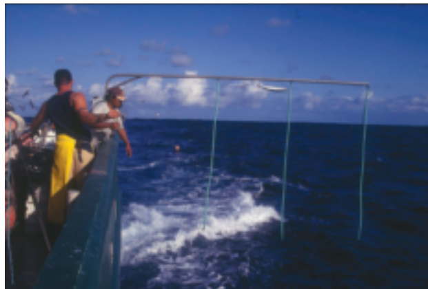
Side-setting and the use of bird curtains has resulted in a 90 to 95 percent reduction bird interactions with the Hawaii longline fishery.
