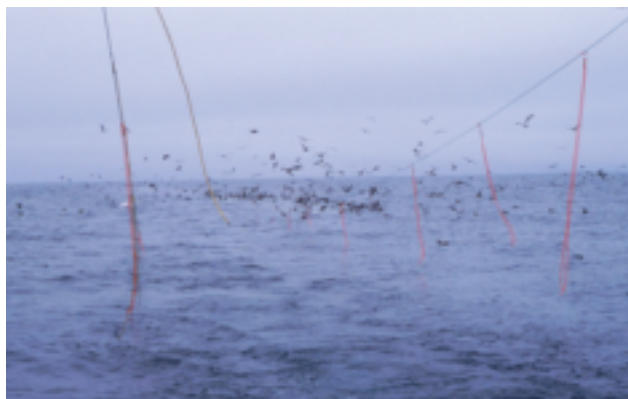
Use of the streamer lines on longline vessels has resulted in an 80 percent reduction in seabird bycatch in Alaska.
